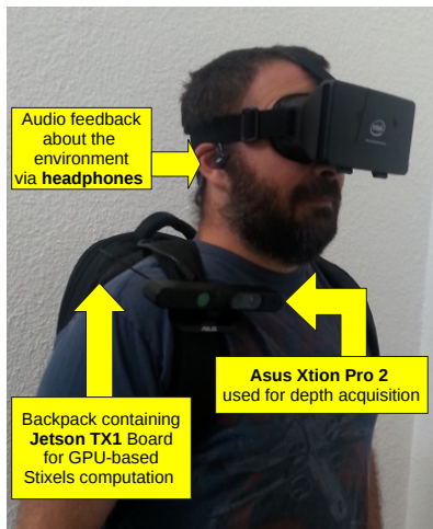
Figure 8: Blindfolded user equipped with the developed prototype system. Computing board is placed inside the backpack and Asus Xtion Pro sensor is attached to its strap in the front. Sound helps the user to avoid detected obstacles.
