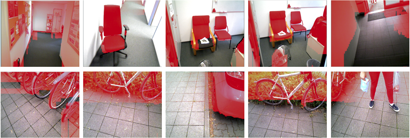
Figure 7: Visualization of our the obstacle detection system algorithm developed for autonomous cars. Stixels-based method was adapted for assisting visually impaired people and tested in indoor and outdoor environments. Detected obstacles are marked in red. Top row: indoors. Bottom row: outdoors.
